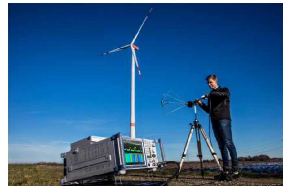
Battery-operated in-situ measurements with the R&S®ESR.
