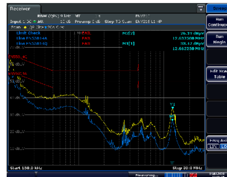
The R&S®ESR performs disturbance voltage measurements up to 30 MHz with quasi-peak and average weighting in a single shot.
